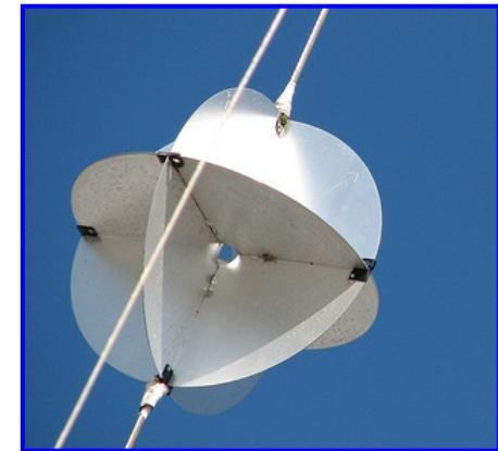
Sailboat Based Circular Trihedral Corner Reflector
